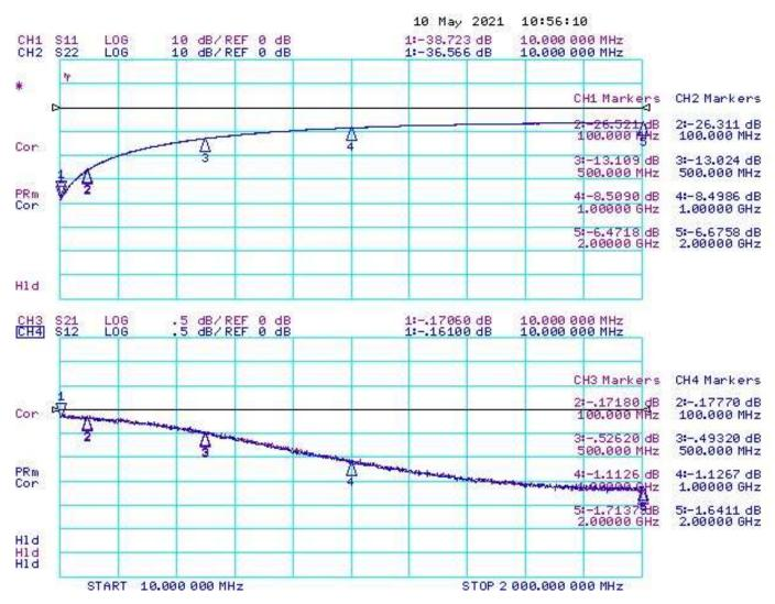
Note: Small Signal data taken without DC Blocking capacitors
