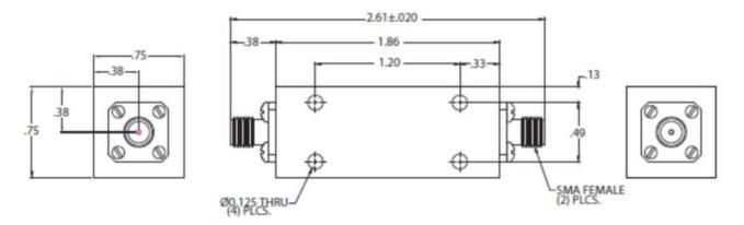
The RFLM-300511QA-392C SMA Connectorized package included input and output DC Blocking capacitors.
